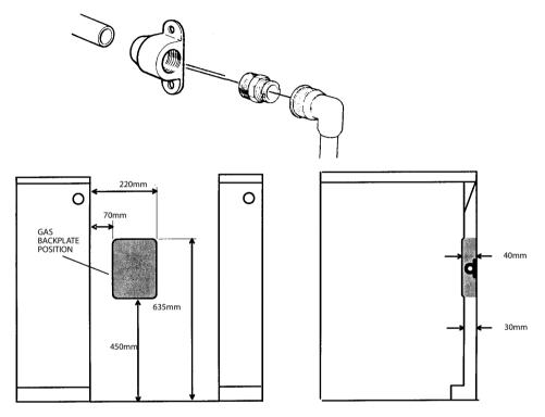
Connection to the cooker should be made with an approved appliance flexible connection to BS 669. A length of 0.9 to 1.25m is recommended. The length of hose chosen should be such that when the cooker is in situ, the hose does not touch the floor.
